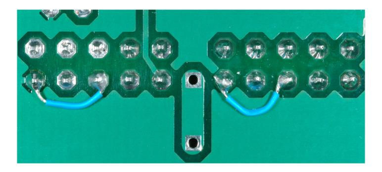
In addition, the spacing between the two headers is a little tight and fitting a pair of ribbon cable connectors may be difficult. Filing the edges of the connectors will free up enough room. Sorry about that.
