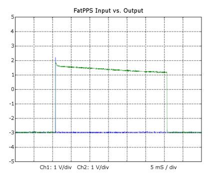
The output pulse is about 30 milliseconds long.
