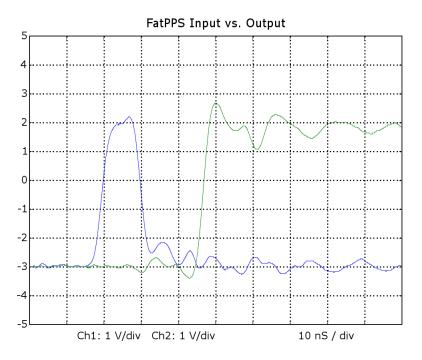
Note that the propagation delay from the rising edge of the input to the rising edge of the output is about 25 nanoseconds. (The transient response of this plot is limited by the 100 MHz digital oscilloscope being used).
