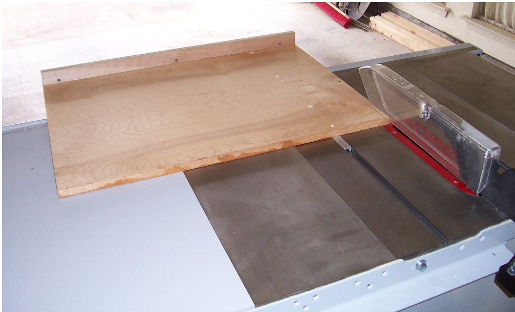
Figure 7 – Panel cutter after slot tune-up. The twist between the panel and the table top is reduced by about a factor of three.
