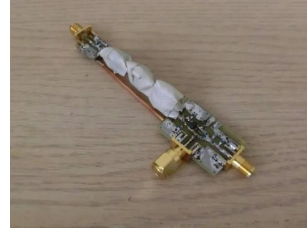
Reflection Bridge (for S11 measurements)
