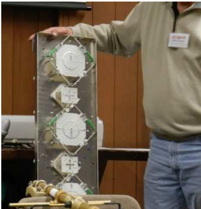
Ellis show the front of a variable-down angle multiband directional cellular antenna
