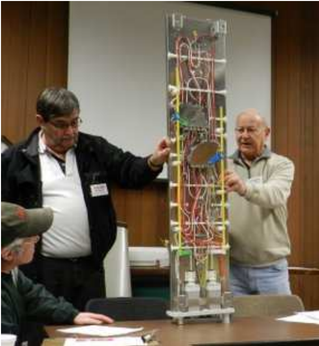
Ellis and Don show the back of the same variable-down angle multiband directional cellular antenna
