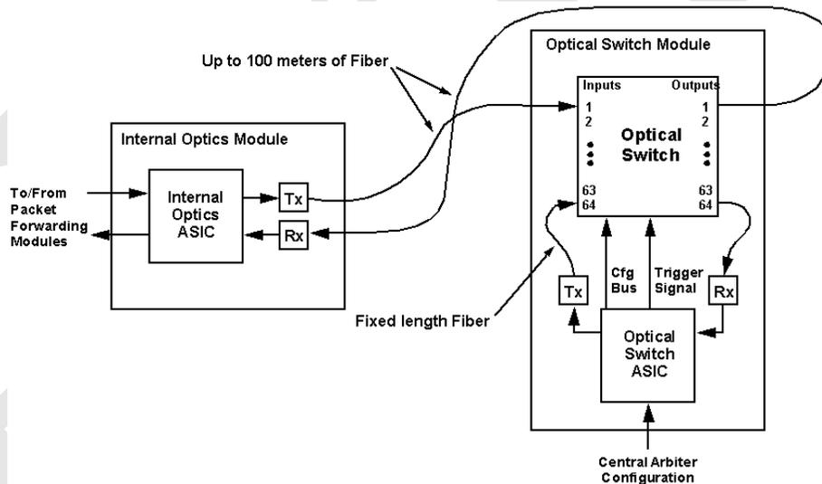
Fig. 2. Fabric synchronization functionality.
