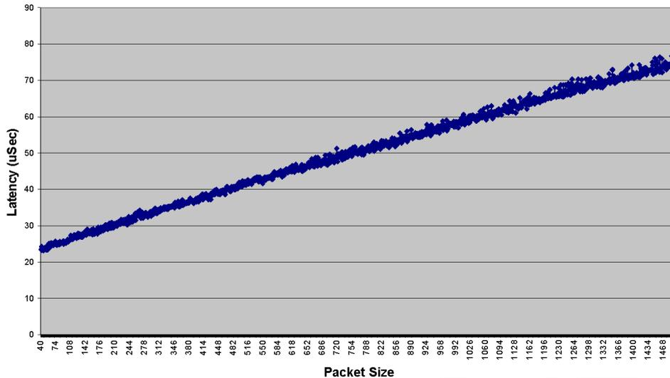
Fig. 5. Minimum latency versus packet size for optical router with 1-Gbit Ethernet interface, with four GbE packetize–depaketize steps.
