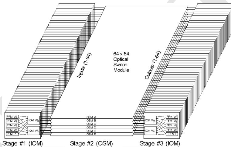
Fig. 1. Chiaro router switch fabric.
