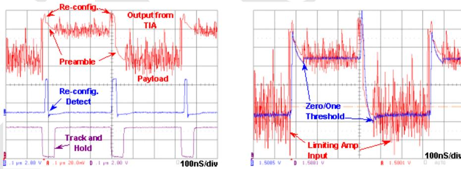
Fig. 3. Example burst receive signal with large chunk-to-chunk power variation.
