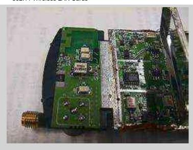
SMA antenna jack and the Toko TDF2A-2450-T bandpass filter. Also shown are the transmit/receive LEDs. The right section is the RF power amplifiers and receive pre-amplifier sections.
