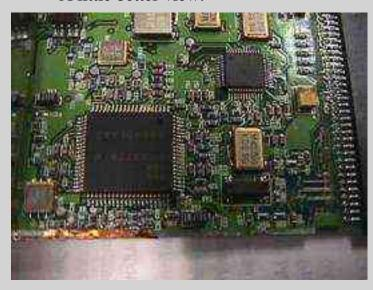
Shown are the HFA3726 400 MHz quadrature IF modulator/demodulator and the HFA3824 direct sequence spread spectrum baseband processor (small IC upper right) and their support components.
