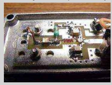
Closeup of the receive pre-amplifier's RF input, showing the shunt inductor and the modified series gate inductor.
