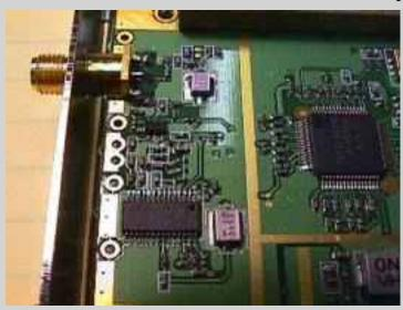
RF power amplifier, standard PRISM2 based hardware.
