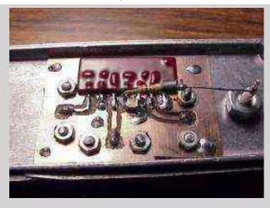
Closeup of the PIN diode module. You can see the bias resistor and ferrite bead floating in the air. The bias line passes through a regular feed-through (non-capacitor). RF connectors are SMA, with the teflon covered pin (ala the 33LNACK), the connectors are also available from Down East Microwave.
