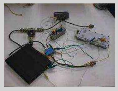
All the modules sorta put together. Please don't use alligator clips, I'm a professional. The male SMA jumper cables are from Down East Microwave.
