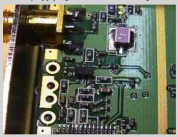
UPG152TA TX/RX switch and the bandpass filter.
