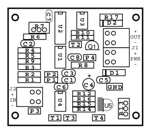
Electrolytic capacitors are cylindrical with radial leads (meaning both leads come out one end). The negative lead is usually marked with a black band filled with minus signs. In addition, this lead is usually shorter than the positive one.
