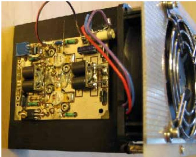
Figure 2: The driver amplifier AN779H mounted on a heat sink with blower. It delivers about 8-10W and it is in-stalled inside a cabinet that houses the TAPR boards Mercury (receiver), Penelope (transmitter), Ozymandias (bus and control) together with the corresponding power supplies.
