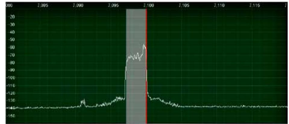
Figure 12: Accumulated spectrum applying the “Peak” function of PowerSDR with a FLEX-5000A as measuring instrument with scaling the same as in Figure 9. The spectrum gives the maxima within the wanted LSB as well as IMD maxima outside; the latter being down by almost 60dB compared to the maximum in-band power density.
