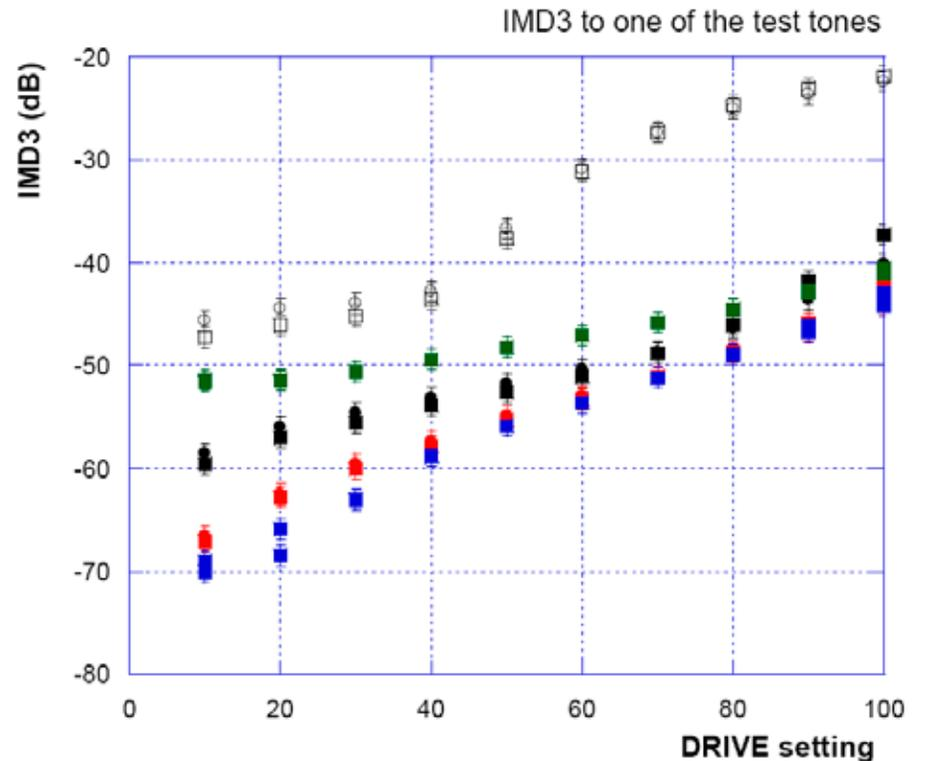
Figure 3: IMD3 for Penelope with driver amplifier as a function of the Drive setting in PowerSDR, which is directly proportional to the output power; Drive=100 corresponds, in this case, to (8-10)W. The colors distinguish the measurements on different bands: black=80m, red=40m, blue=20m, green= 15m, open black symbols=160m (see text). Really excellent results are obtained for settings below about Drive=50 (about 4W PEP) and for the bands 80 to 15m.
