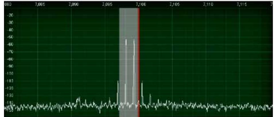
Figure 10: Spectral display (Panadapter) of the PowerSDR software measuring the overall emission of Penelope and the subsequent driver and PA CCI kits at about 50W PEP at 7.1 MHz: vertical scale 10dB per division, horizontal 1kHz. IMD3 is down by more than -50dB compared to one of the test tones.
