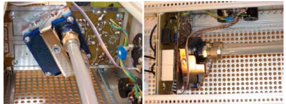
Figures 5: Left: The AN758 amplifier board with the cooling system installed. The front plate is on the right. The bracket next to the water pipes fixes the heat exchanger to the copper plate to which the transistors are mounted. Right: A different view of the cooler.
