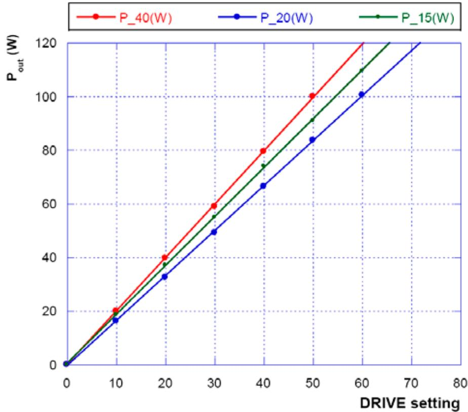
Figure 9: Power output for three bands, 40, 20, 15m as a function of the Drive setting in PowerSDR for Penelope + driver + PA verifying the linear relation between the two and in addition, demonstrating that the 100W level can be reached with this combination with Drive below about 60 where IMD3 of Penelope + driver are below -50dB.
