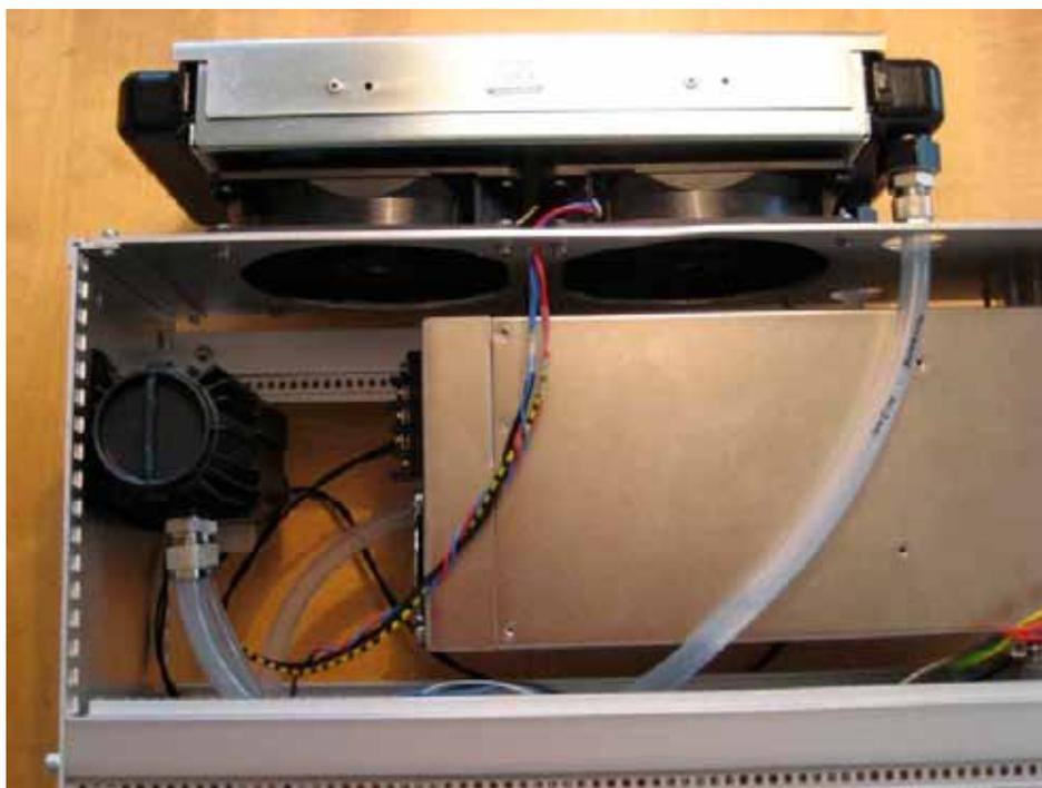
Figure 6: The rear part of the 19-inch cabinet with the water-to-air heat exchanger with two blowers and the water pump in the left corner. The large metallic box to the right is a 50V, 750W switching power supply.
