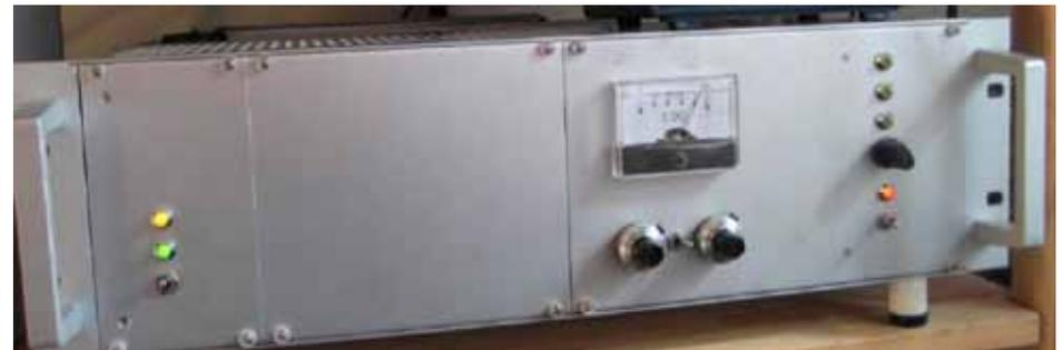
Figure 7: Front view of the water-cooled amplifier. The AN758 amplifier is mounted on the right side. Behind the left side of the front plate, a 13.8V power supply is mounted. The instrument shows the total collector current of 8A. The amplifier can be switched between class-AB and class-A mode of operation; the operating points are adjusted with the two 10-turn Heli-potentiometers below the instrument.
