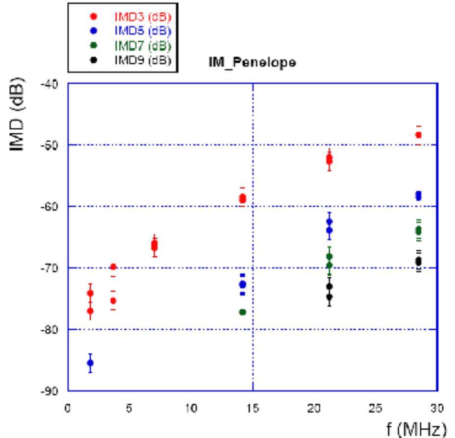
Figure 1: The various orders of intermodulation distortion IMD as measured at 400mW PEP output power on the TAPR Penelope module. IMD is given in dB below one of the two test tones used (not to PEP). Several measurements have been conducted. The error bars are based on estimated accuracy and reproducibility. Because of their small amplitudes, the higher IMD orders could not be measured at frequencies below about 10 MHz.
