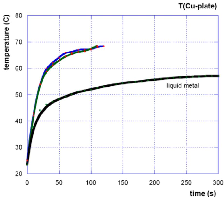
Figure 8: Temperature of the copper plate the PA transistors are mounted to for two different materials used for heat transfer improvement. The upper curve corresponds to the standard silicon paste (Thermaflow), the lower one to liquid metal.
