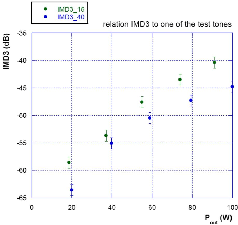
Figure 11: Overall IMD3 as a function of PEP output power for Penelope + driver + PA for two bands, 15m (green) and 40m (blue).
