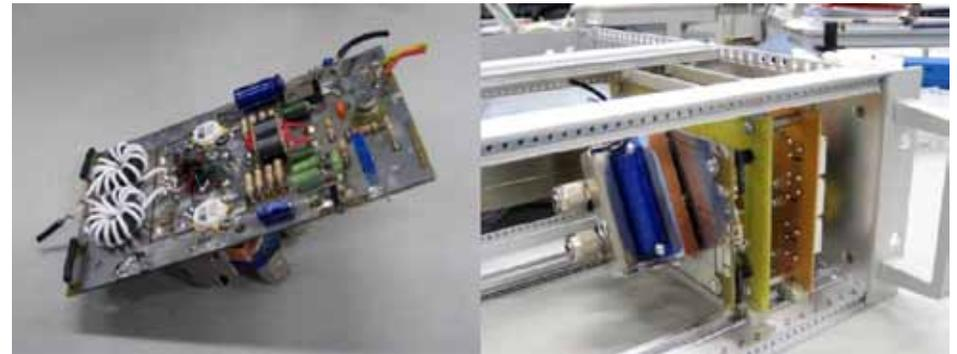
Figures 4: Left: The AN758 amplifier board with the transistors in close contact with the water cooled copper plate of the processor heat exchanger. Due to the limited size of the cooler of 63x63mm<sup>2</sup>, it had to be mounted diagonally. Right: The amplifier board is connected with two other EU-standard boards that carry the low pass filters and some control units; the module has been built up as plug-in unit to a 19-inch cabinet. In this picture, the front plate is still not installed.
