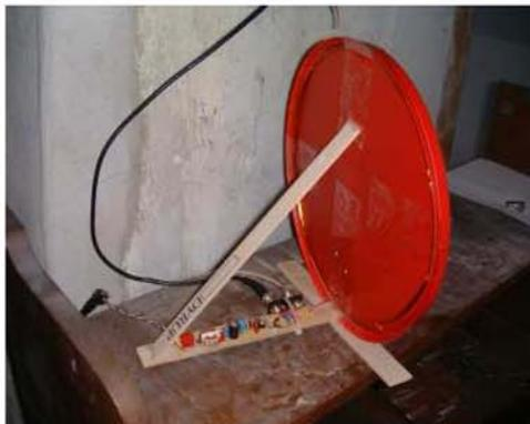
Figure 6. \$20 homebrew loop antenna
