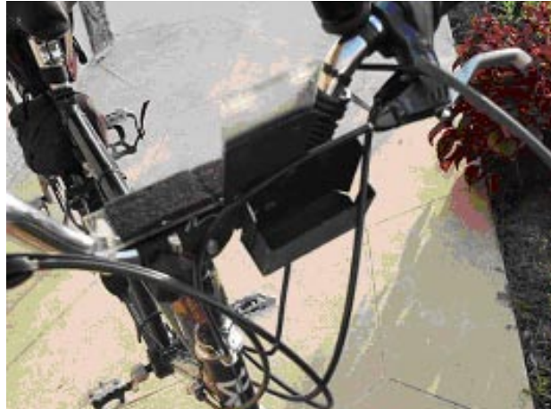
Figures 7 and 8. A sheet metal battery pack holder counterbalances the radio on the handlebars.
