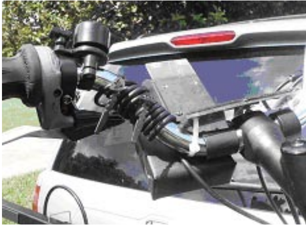
Figures 7 and 8. A sheet metal battery pack holder counterbalances the radio on the handlebars.
