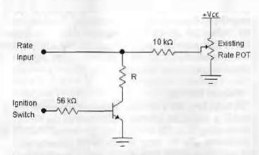
NOTE: you must insert a new 5k resistor in series with the existing RATE pot input so that the new circuit can share the input as shown.
