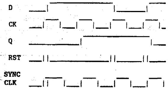
Next, the synchronized clock is applied to one input of EXCLUSIVE-OR gate 2, with the data applied to the other input. The output is Manchester encoded data suitable for JAS-1.
