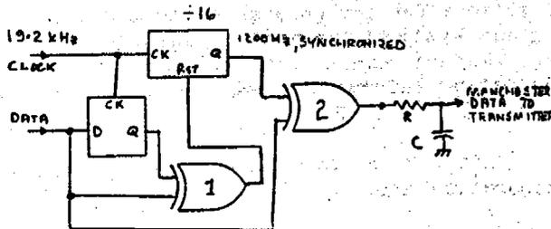
The TNC-provided clock of 19.2 kHz is 16 times the desired 1200 Hz clock signal. So, we apply the clock to a divide-by-16 counter and voila! we have our 1200 Hz clock.
