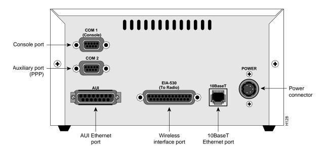
Figure 1-3 **Router Rear Panel**
