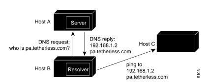
To take advantage of DNS, you must identify the domain name of the router you are configuring and the IP address of the name server you want to handle DNS requests. You can define multiple name servers to balance DNS requests.
