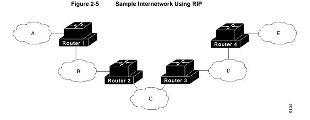
Table 2-5 illustrates the routing table for a datagram travelling from a host on Network C to hosts on other networks within the internetwork. For example, to send a datagram from a host on Network C to Network E, the datagram travels across three hops:
