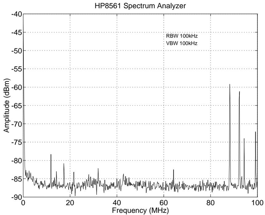
Figure 39: Noise spectra of DSP CARD 4 when in metallic box, and all the wires are bypassed.
