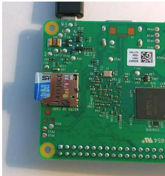
*Figure 3: SD Card Inserted into rPi*
