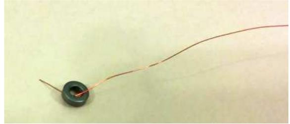
*Figure 22: Winding Toroid 2*
