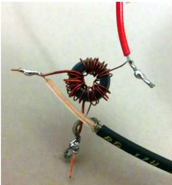
Figure 27: Soldering Toroid
