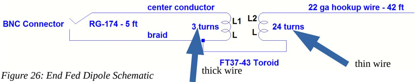
Figure 26: End Fed Dipole Schematic
