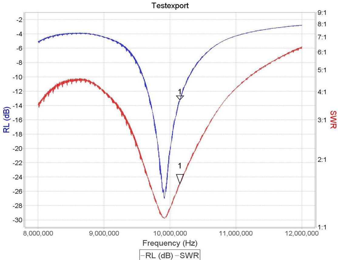
Figure 31: Antenna Response - Raised 6'
