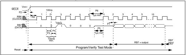
FIGURE 5-3: INCREMENT ADDRESS COMMAND (PROGRAM/VERIFY)
