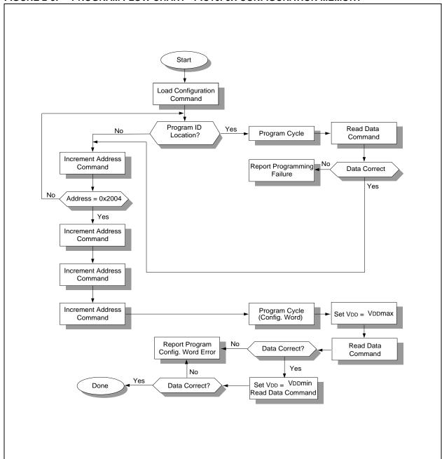
FIGURE 2-3: PROGRAM FLOW CHART - PIC16F8X CONFIGURATION MEMORY
