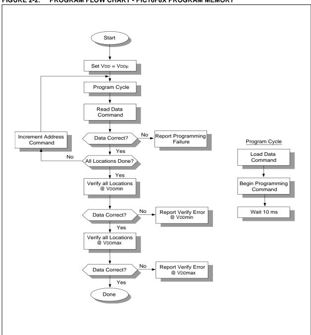
FIGURE 2-2: PROGRAM FLOW CHART - PIC16F8X PROGRAM MEMORY
