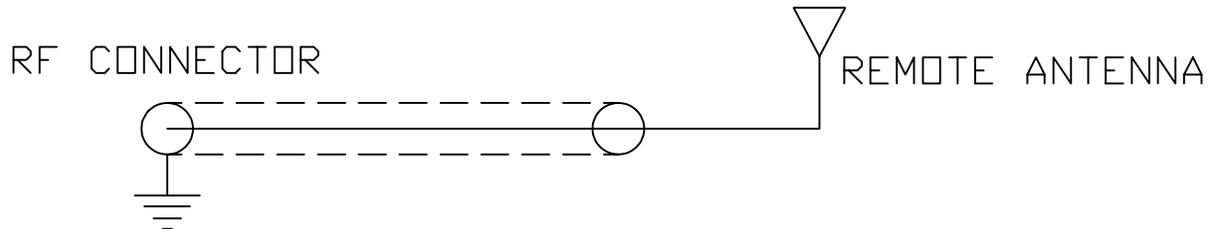
Coaxial cable supplies +5V @ 15 mA to antenna/preamp. 1.57542 GHz signal returns to the sensor board.
