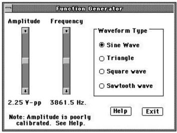
Figure 2 - Function Generator panel
