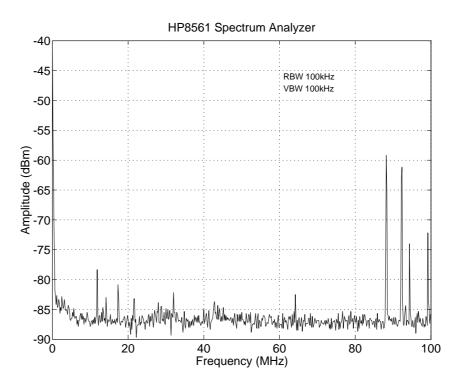
Figure 39: Noise spectra of DSP CARD 4 when in metallic box, and all the wires are bypassed.
