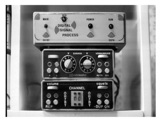
Figure 31: OH7BY's Satellite station with DSP CARD 4. At the top is DSP in a box, below is 2m transmitter and the lowest box is a 70 cm receiver. Both radios have previously been auto radiophones.
