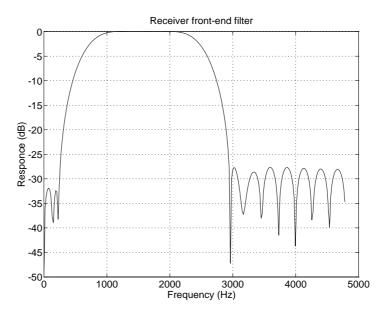
Figure 23: Amplitude response of the input bandpass filter
