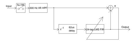
Figure 19: Block diagram of the QRN reductor
