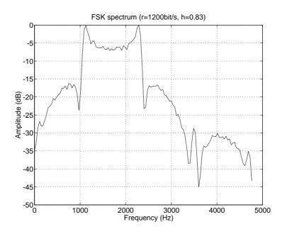
Figure 21: Spectrum of 1200 bit/s Bell 202 FSK-signal
