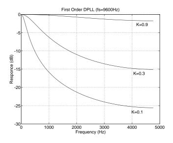
Figure 24: Phase response of the first-order DPLL with varying loop gains Locking range of the loop is defined as
