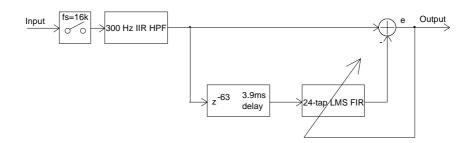
Figure 18: Block diagram of the QRM reductor
