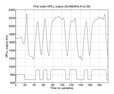
Figure 25: 1200 bit/s Bell 202 FSK-signal and demodulated result
