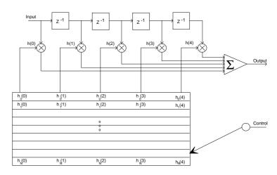
Figure 30: Polyphase filter structure
