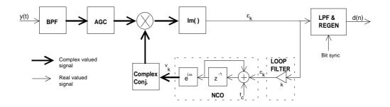
Figure 22: FSK demodulation with digital phase-locked loop
