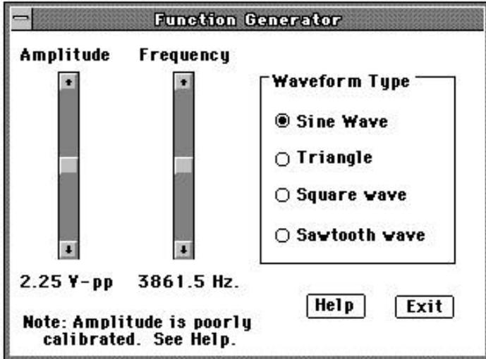
Figure 2 - Function Generator panel
