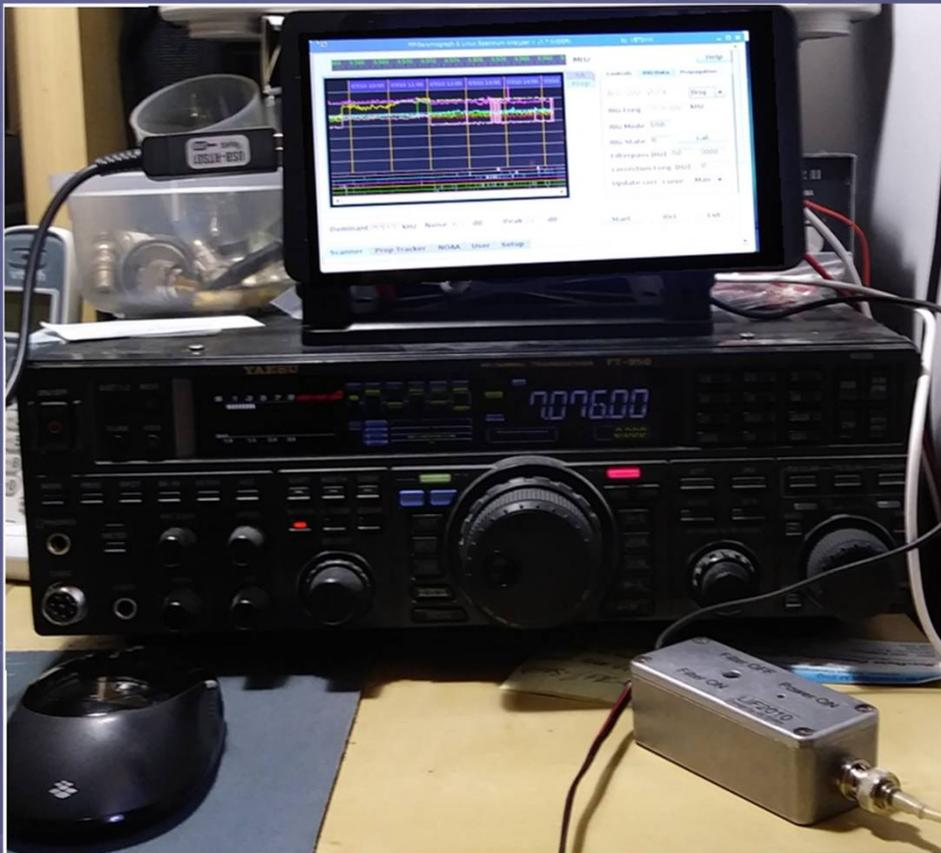
5V 2A power is supplied via a 12V car power adaptor. The LIF interface (cast metal box) requires 12V/10mA power.
