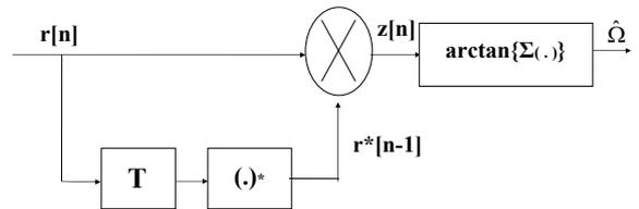
Fig. 1. Block diagram of the single-delay multiplication based frequency estimator.
