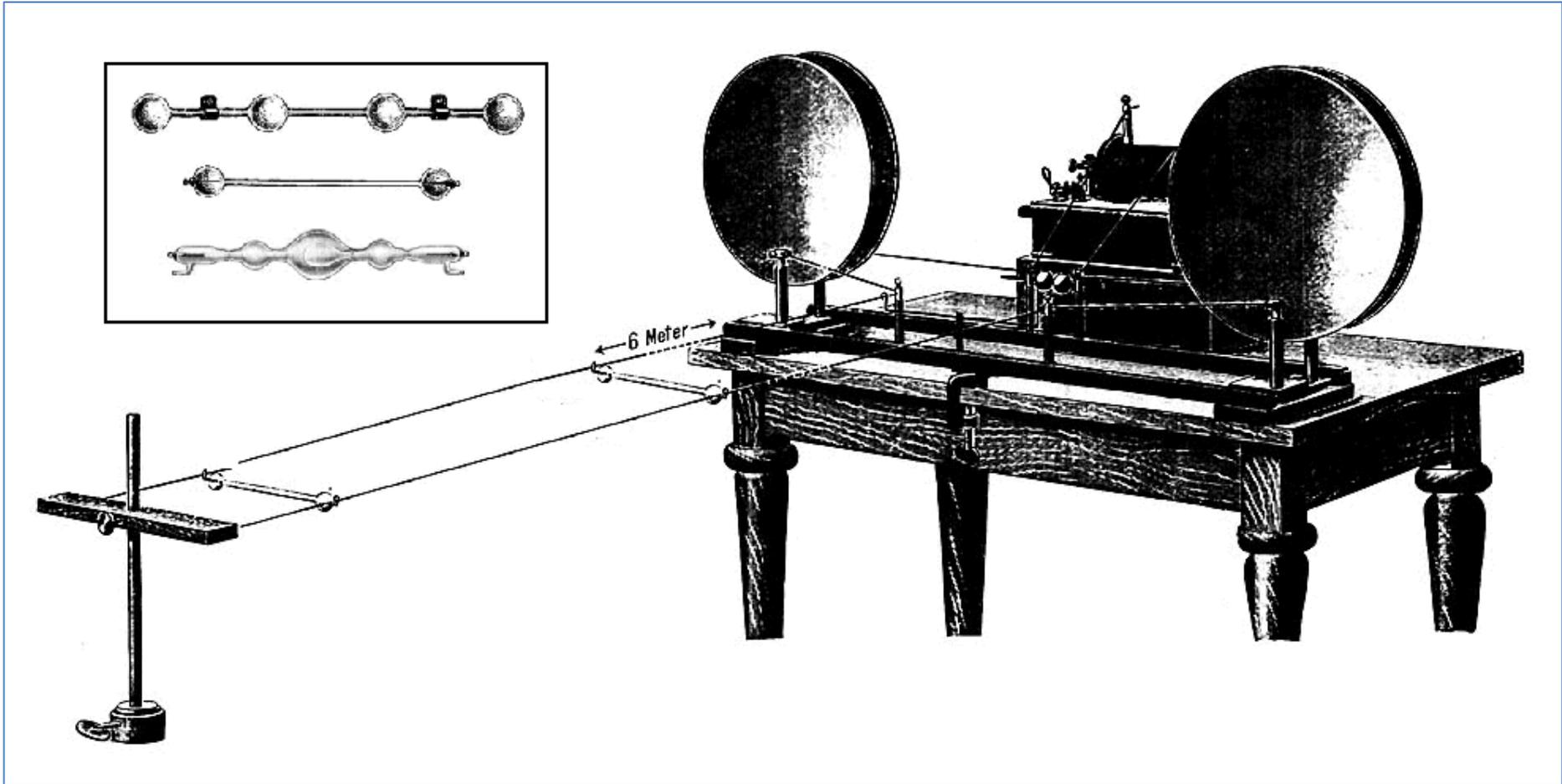
Lecher line: High SWR by design! Light bulb is used to probe for voltage nodes.
