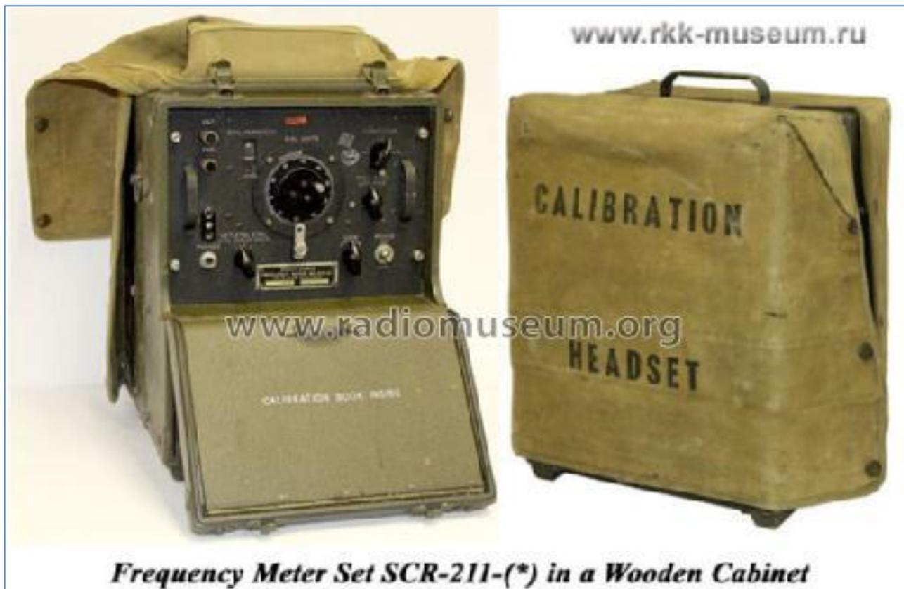
Used to be used a lot for FMTs. Could get within about 10 Hz on a good day.
