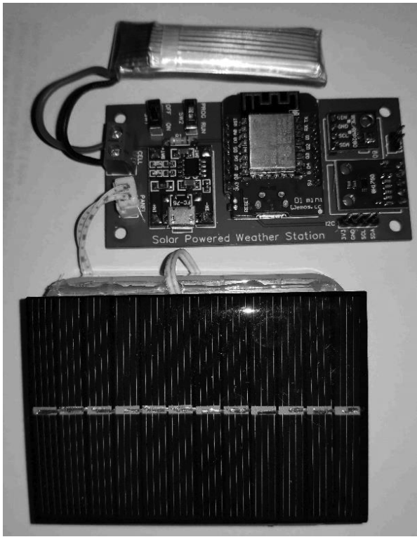
Figure 2 Single Board Version with Solar Panel and LiPo Cell
