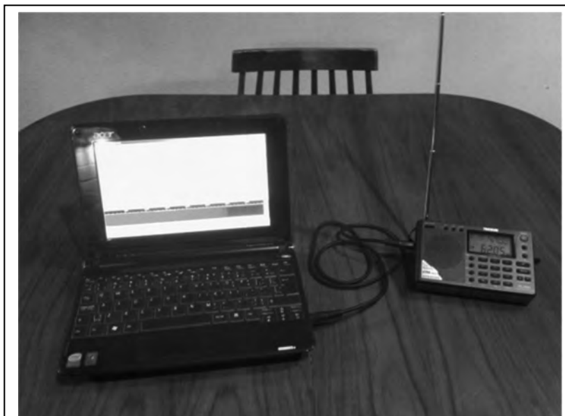
Figure 2: Typical equipment needed to receive and decode VOA adiogram broadcasts is a portable shortwave radio and a notebook PC, with a patch cord feeding audio from the former to the latter. Appropriate software is also necessary.
