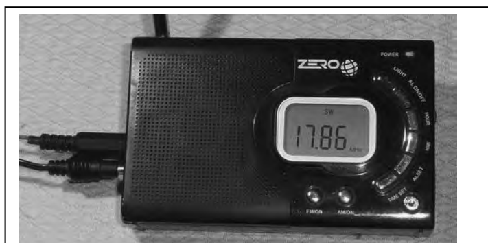
Figure 8: This $25 radio in Germany provided audio for a successful decode of VOA Radiogram text.
