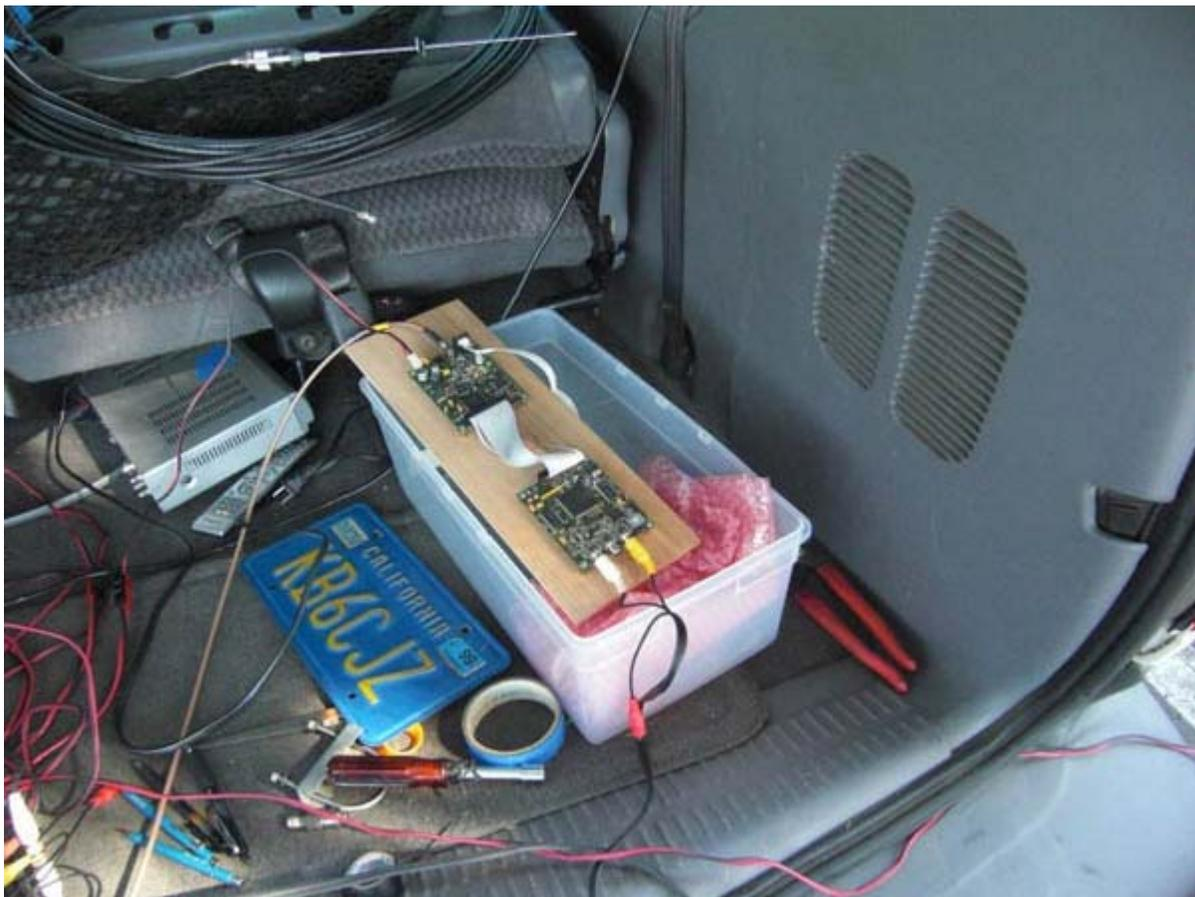
**Figure 11 – DATV DVB-S 1 mW Transmitter for 1.2 GHz**
