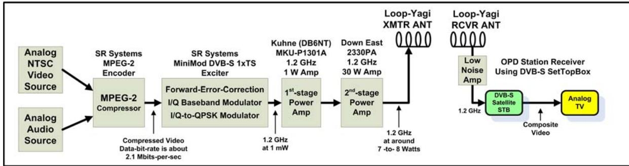
**Figure 21 – Block Diagram of DVB-S Transmitter and Receiver for DATV Field Tests**
