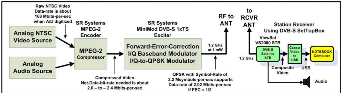
**Figure 1 – Block Diagram Showing DATV Exciter being Tested**
