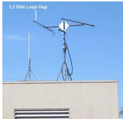
**Figure 23 – 1.2 GHz Loop-Yagi receiving antenna on roof of OPD**
