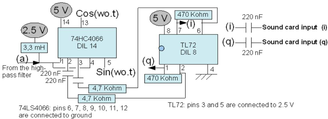
The system below supplies two signal in quadrature at a frequency  $f_0$  equal to the quarter of the frequency of the crystal oscillator (i.e. here:  $14.31818/4=3.579545$  MHz). These signal are not, strictly, sinusoidal ( $\text{Cos}(\omega_0 t)/\text{Sin}(\omega_0 t)$ ) but rather TTL signals, so with harmonics which are not annoying because removed downstream (either by the TL72 amplifier and the anti-folding filter of the sound card in RX or by the low-pass filter in TX).
