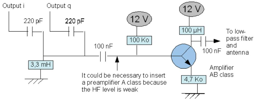
The transistor used could be a 2N2219
