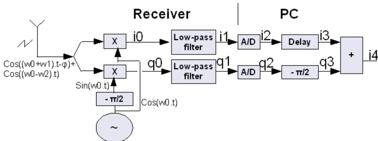
Note : the system being supposed linear, the USB signal  $(\cos((w_0+w_1).t-\varphi))$  can be considered independently of the LSB signal  $(\cos((w_0-w_2).t))$ .
