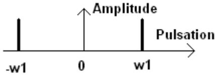
The AF signal to be transmitted can be either a PSK31 signal, a pure carrier (« Tune »), a CW signal or a phone signal. It will be supposed, here, an AF carrier of  $f_1$  frequency and  $w_1$  pulsation (with  $w_1 = 2 \times \pi \times f_1$ ) written  $y = \text{Cos}(w_1.t)$ .
