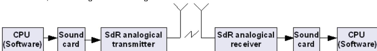
The sound card is the digital  $\rightarrow$  analogical interface (in reception) or the analogical  $\rightarrow$  digital one (in transmission)
