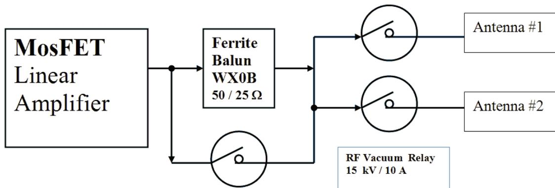
Drawing 2. Principle of stacking.
