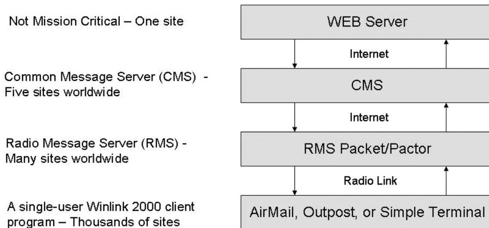
In this case the bottom of the stack is a simple user client such as AirMail, Outpost, or even a simple terminal. These client programs provide an interface to WL2K without the complications of Paclink and separate SMTP/POP3 email client programs.
