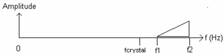
The frequency relocation will be done as previously but the 0 Hz of the frequencies band will be shifted compared to the position  $f=0$  Hz. All the frequencies being shifted to the high notes, the listening will be at the best unpleasant and the at worst impossible. Hereafter, it will be found a diagram of this relocation.
