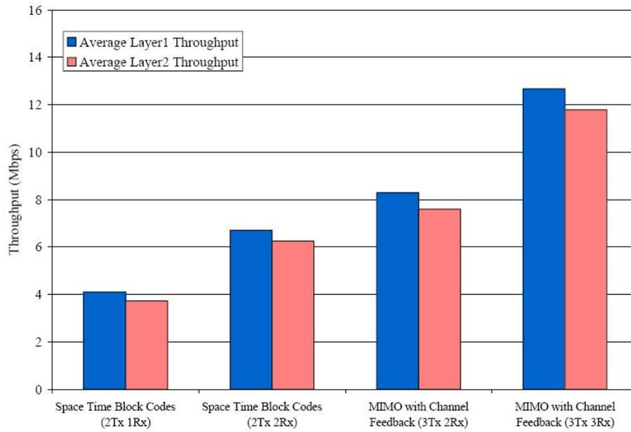
Figure 5 Average throughput per 5 MHz carrier for 802.16d system with enhancements
