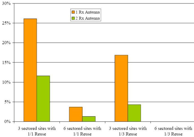
Figure 3 Percentage of cell area with data rate less than 1.5 Mbps
