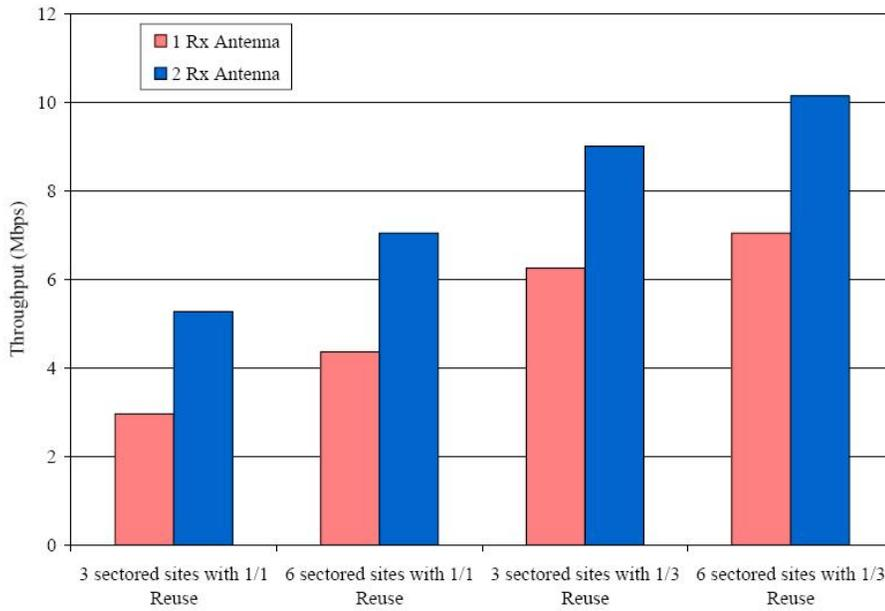
**Figure 2 Average throughput over an entire cell per 5 MHz carrier for 802.16d system under various frequency reuse and sectorization configurations**
