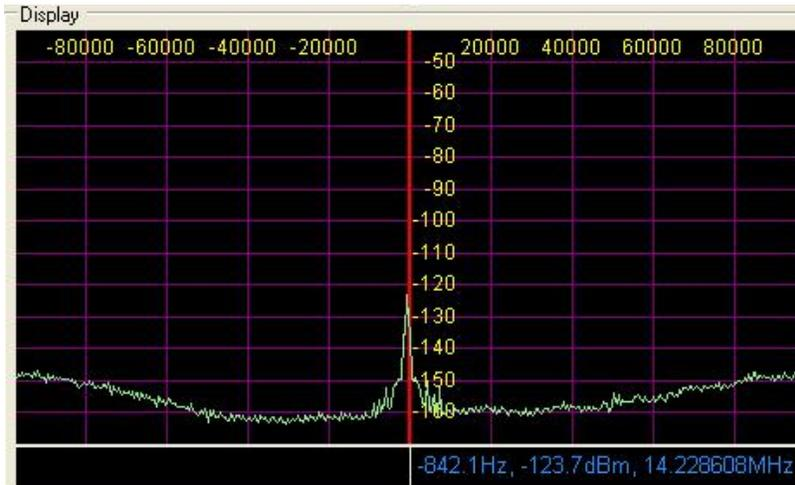
Figure 4 – Wolfson WM8785 @ 192kHz sampling rate
