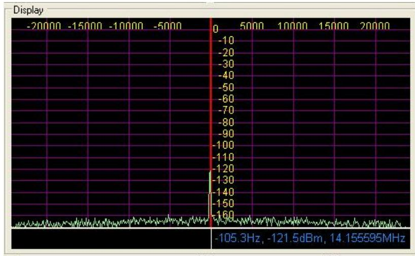
Figure 7 – AK5394A @ 48 khz Sampling
