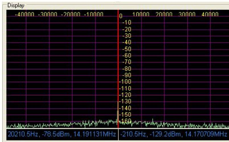
Figure 8 – AK5394A @ 96 khz Sampling
