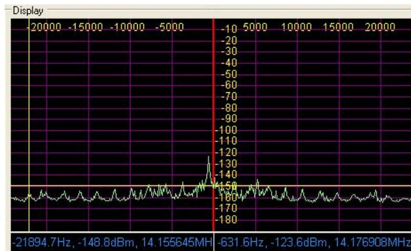
Figure 3 – Cirrus Logic CS5381 @ 48kHz Sampling
