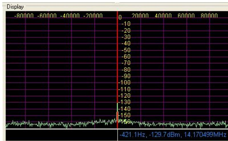
Figure 9 – AK5394A @ 192 khz Sampling
