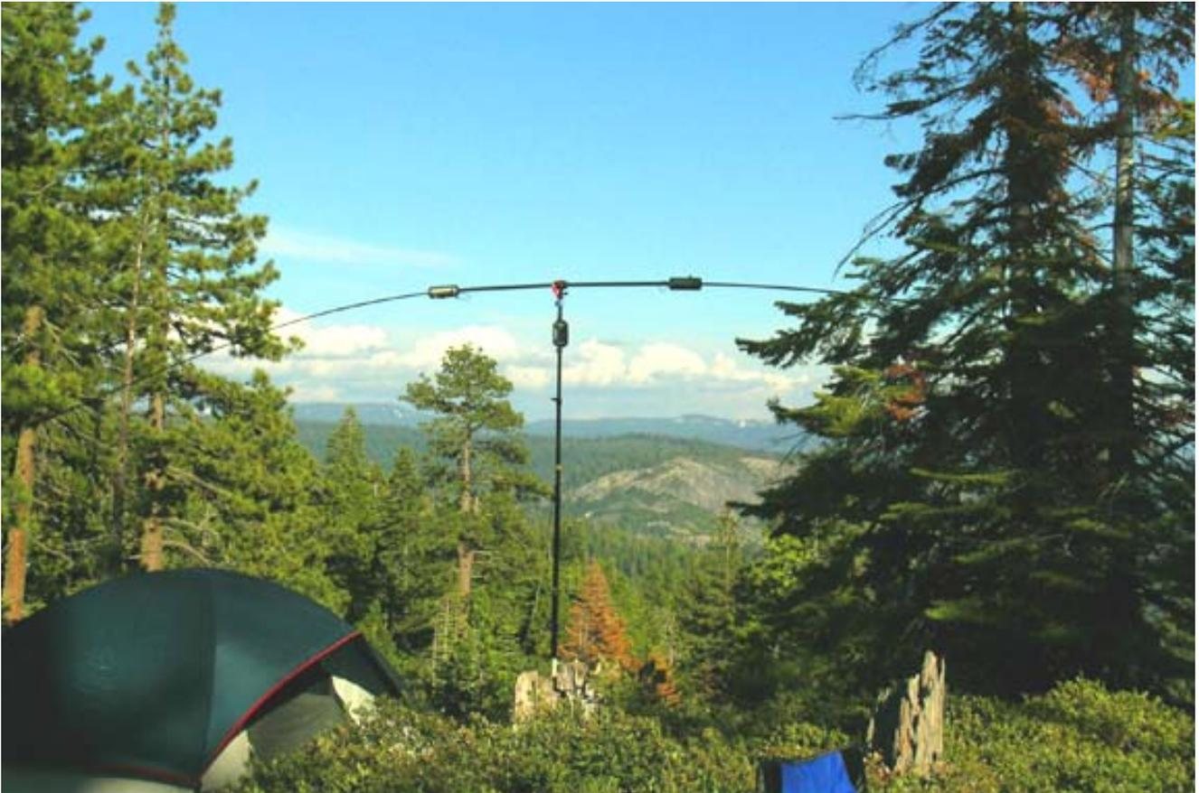
Fig.2 The W3FF 80M Commercial Buddipole was only 11ft. off the ground for NVIS propagation.
