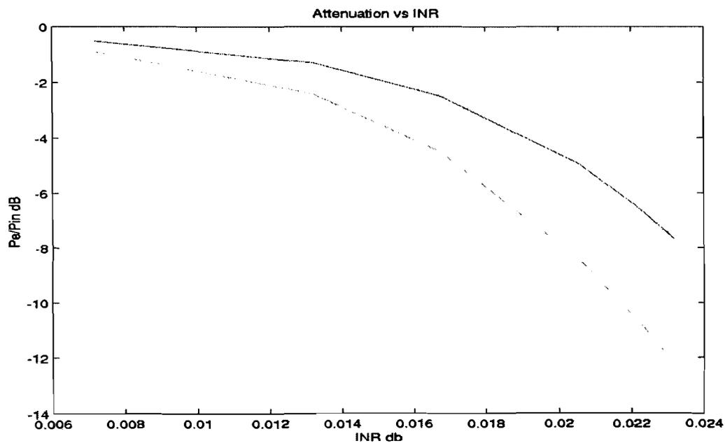
**Figure 3: Simulation results of adaptive interference cancellation, Attenuation vs INR. The results show that constraining the bandwidth of the reference signal, the suppression of RFI improves with SNR**
