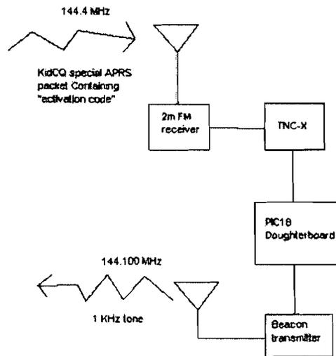
Figure 4: KidCQ Prototype Device Block Diagram
