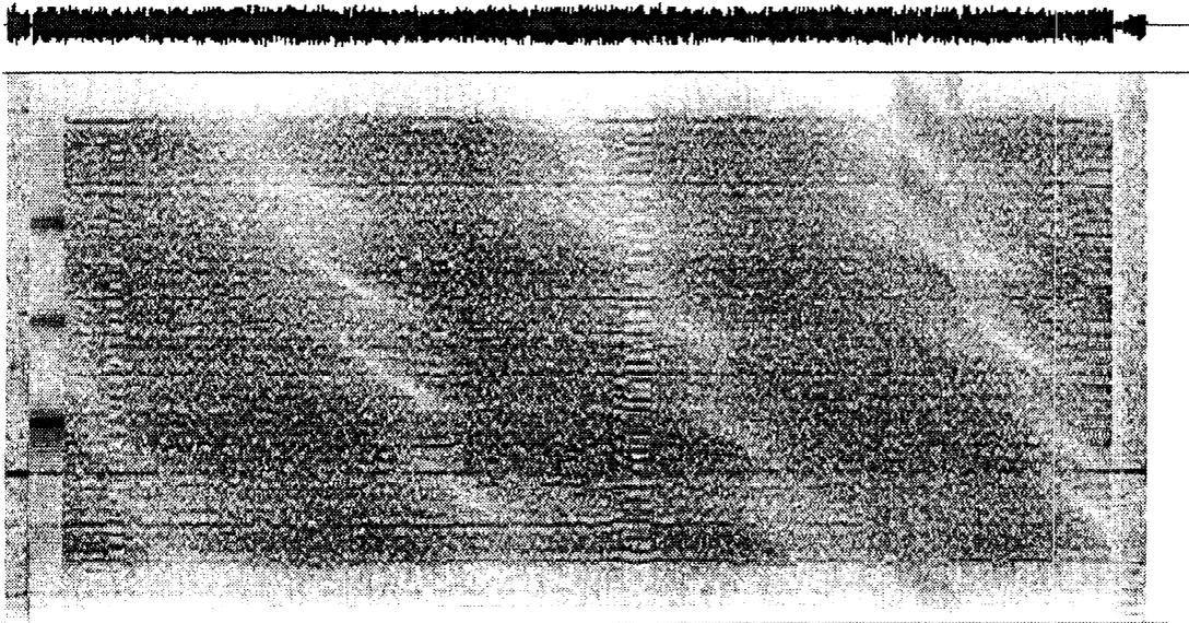
Fig 1 Off air spectrogram of M36 modem
