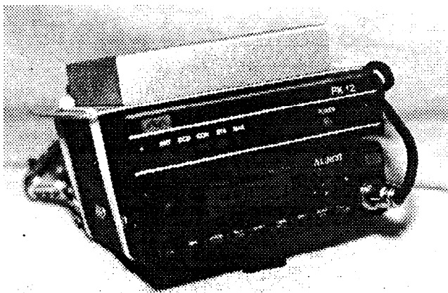
Figure 3. This photo shows a typical PACSAT mobile status/position reporting station. It consists of a 2 meter FM radio, a GPS unit and a slightly modified TAPR-2 compatible TNC.
