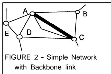
Consider the simple hypothetical network shown in Figure 1. Suppose that node-ops want to convert the link between nodes A and C to a backbone. Technically, its not difficult to do that. A second TNC, a second radio, and (often) a second antenna at each end is about all it takes. Without changing the user frequencies at either end, the result is shown in Figure 2. The heavy line represents the backbone link.
