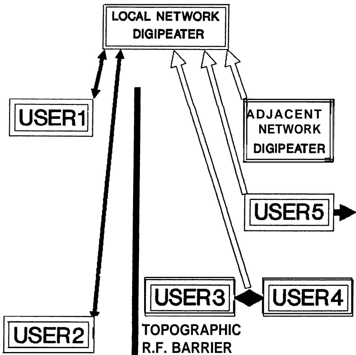
Distant signals from adjacent digipeater direct users 3 & 4, and DX'er 5, cause local digipeater to hold off all output transmissions **until** channel is clear.
