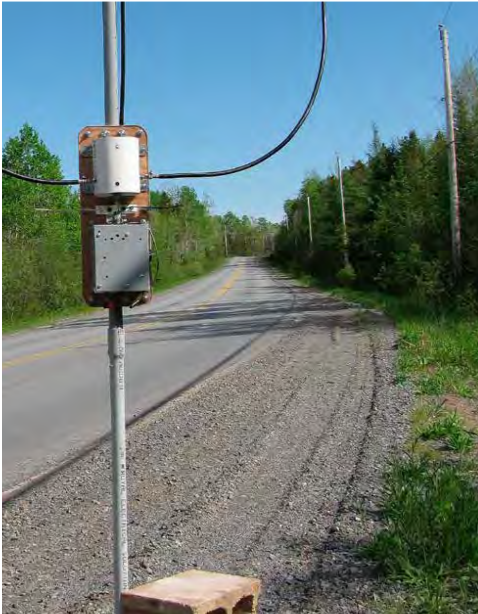
Picture 1. Small Magnetic Loop Antenna with Autotuner
