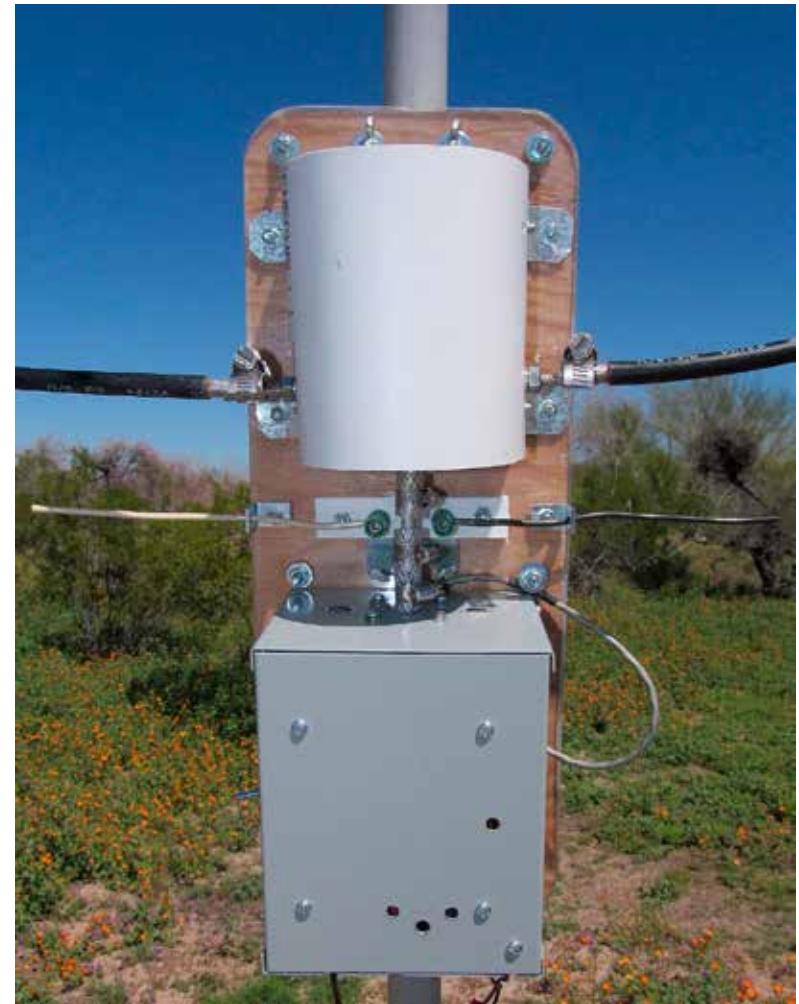
Picture 2. Autotuner - Sampling Antenna Below Variable Capacitor Protector
