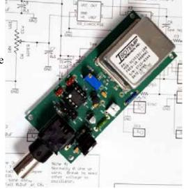
that small OCXOs can have a surprisingly high power draw on startup of 800 ma or more. This reduces quickly to a steady-state current of about 200 ma. If the power supply provides more than about 12 volts, the 7805-type voltage regulator provided with the kit will require substantial heat sinking and possibly replacement with another device. Lower supply voltages will keep things cool(er).
