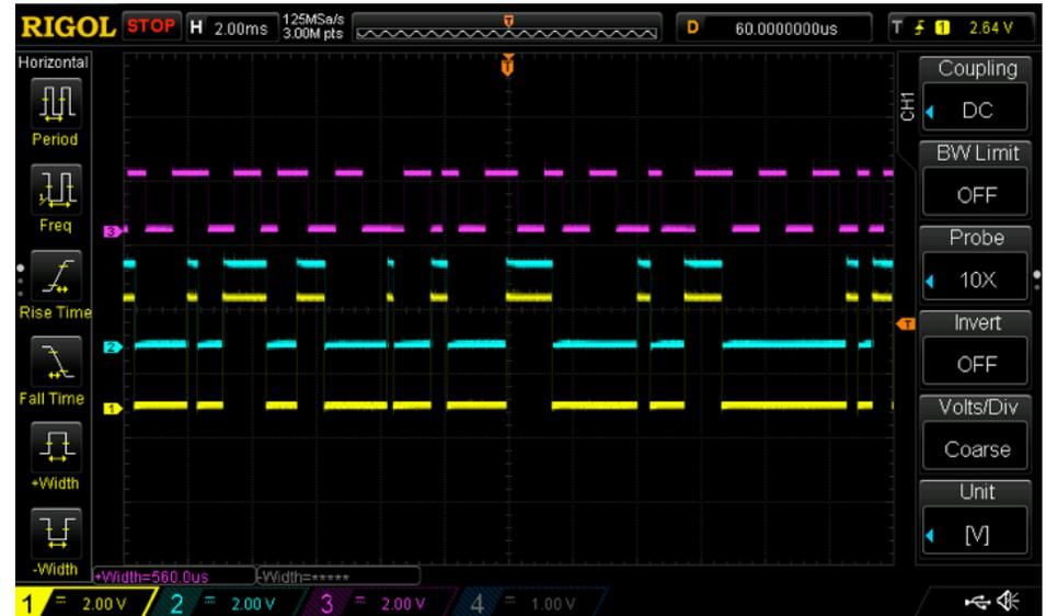
It is obvious from the magenta trace that the system is flailing wildly but failing to sync to the noise, as it should. The next trace shows the last data and first flag at the end of an AX-25 packet with the same setup, and clearly the bit reading is synchronized near the middle of each bit.
