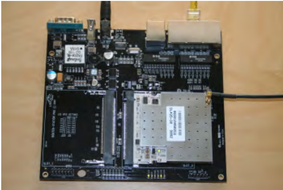
Doodle Labs DL435-30 miniPCI card in Ubiquiti RouterStation Pro
