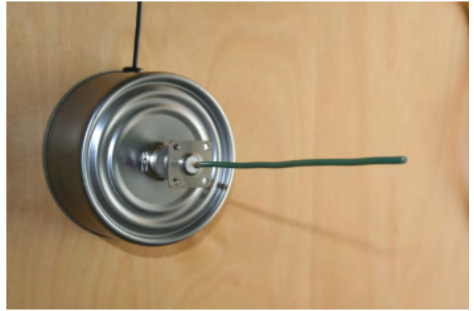
Homebrew quarter-wave 70-cm antenna on a large tuna fish can
