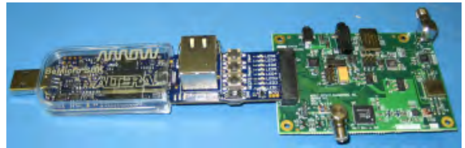
A complete SDR receiver: UDPSDR-HF2 SDRstick paired with BeMicro SDK
