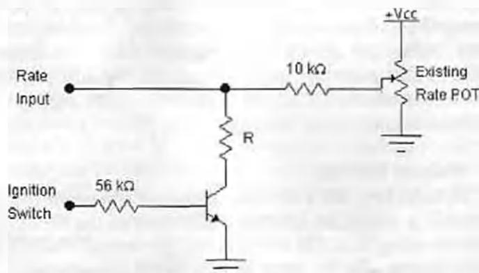
NOTE: you must insert a new 5k resistor in series with the existing RATE pot input so that the new circuit can share the input as shown.
