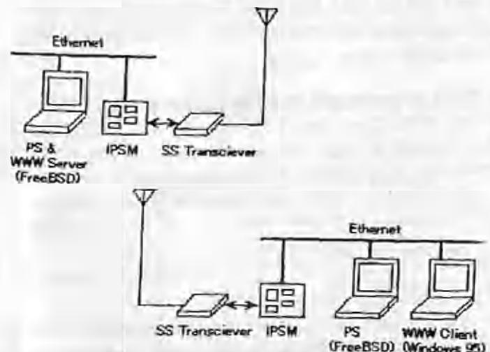
Figure 1. System configuration
