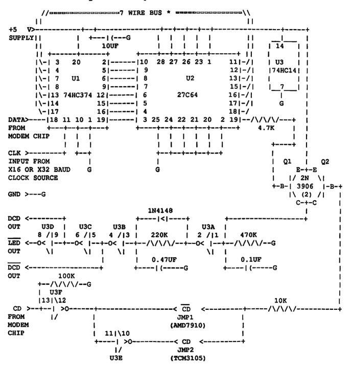
NOTE: Only JMP1 OR JMP2 installed NOT both! \* BUS wire connections are in order vertically. Top pin goes to top pin bottom pin goes to bottom pin etc.
