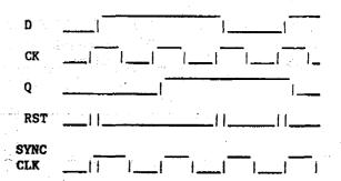
Next, the synchronized clock is applied to one input of EXCLUSIVE-OR gate 2, with the data applied The TNC-provided clock of 19.2 kHz is 160 times the to the other input. The output is Manchester en-
