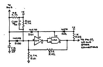
This modification is more complex than Fix #1 and detailed instructions are not provided here. Basically, you have to cut the power traces going to U1 and U3 and jumper around these ICs to provide power to other ICs that are powered by the +5 volt bus after it passes through ICs U1 and U3. Then, add the resistors, capacitors and diodes called out in the parts list below. These are labelled R100-R103, D100-D102 and C100 in the schematic above.
